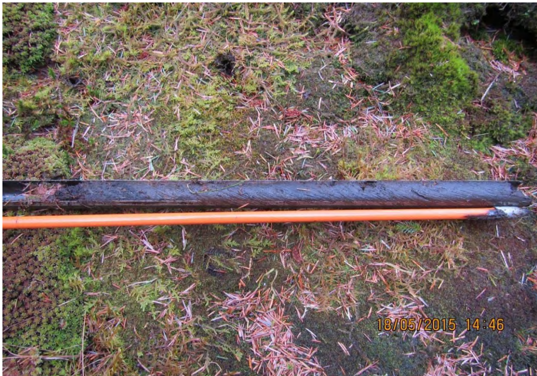
Photo 1 Example of peat probe and core showing a very small thickness of acrotelm in ground below forest canopy.
